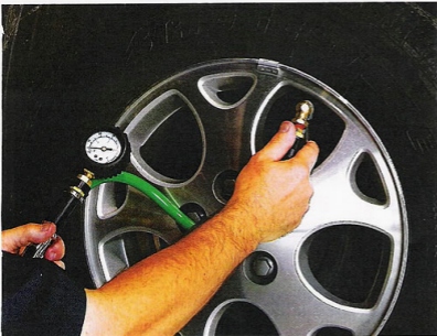
In auto pneumatics, green has become the universal color to designate nitrogen equipment: hoses, tanks, even sometimes valve stems. Regular-air top-ups are harmless, but the nitrogen purge process has to be done over.
